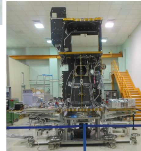
S3B Platform undergoing electrical integration at Platform Responsible facilities in Rome (I)
