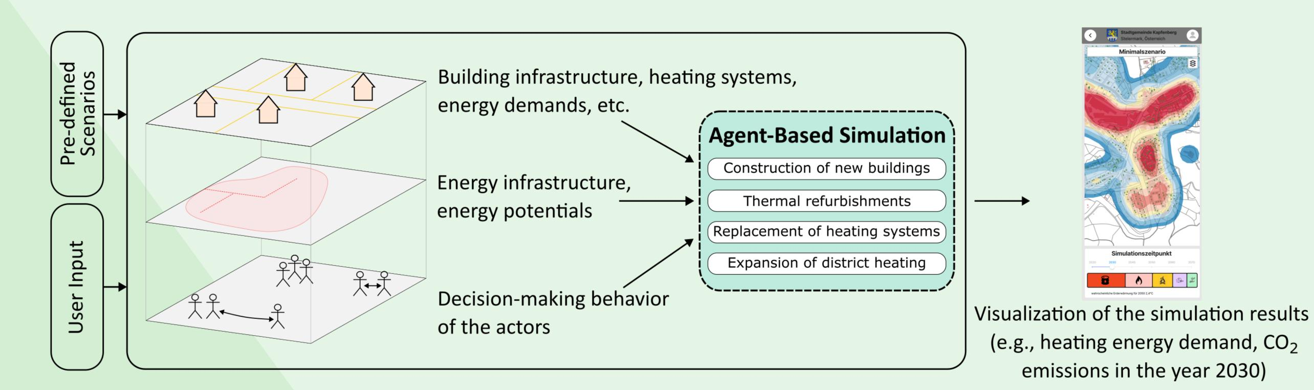
Methodologically, an agent-based simulation model is used to analyze and evaluate transition scenarios for the regional heating and energy transformation
