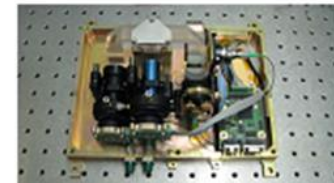
Terminal for Small Satellite Applications (RUAG) Optel- \mu pulsed laser transmitter, optical fibre amplifier and micro pointing assembly
